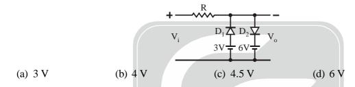
51. Draw the output waveform for a sinusoidal of amplitude 20V. (Assume Ideal diodes)
