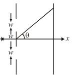
The intensity of the interference pattern, measured on a distant screen, at an angle  $\theta = n\lambda/w$  to the *x*-axis is
