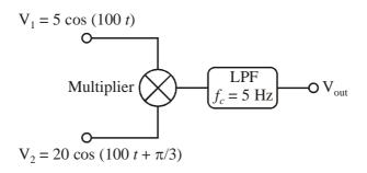
If the roll-off frequency of the LPF is  $f_c = 5$  Hz, the output voltage  $V_{out}$  is (a) 5 V (b) 25 V (c) 100 V (d) 50 V
