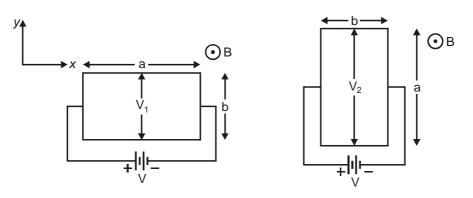
If the Hall voltage across the y-direction in the two cases satisfy  $V_2 = 2V_1$ , the ratio a:b must be (a) 1:2 (b)  $1:\sqrt{2}$  (c) 2:1 (d)  $\sqrt{2}:1$
