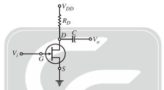
If the drain D-source S saturation current  $I_{DSS}$  is 10 mA and the pinch-off voltage  $V_p$  is -8V, then the voltage across points D and S is
