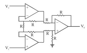
The op-amp are ideal and all resistors are of equal value R. The gain, defined as the output voltage  $V_0$  divided by the differential input voltage  $V_1 - V_2$ , is equal to
