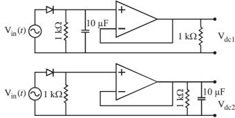
In the DC output voltage of the top circuit has a value  $V_{dc1}$  and the bottom circuit has a value  $V_{dc2}$ , then which of the following statements about the relative value of  $V_{dc1}$  and  $V_{dc2}$  is correct?
