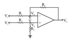
In the above given op-amp figure. Find the value of output voltage in term of  $V_1$  and  $V_2$ . Soln. By the VGP condition  $V_p = V_n = V$ .
