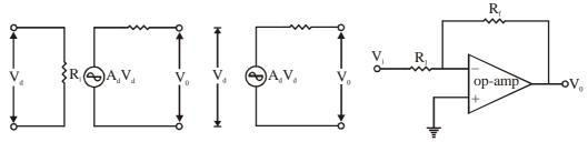
**Inverting Amplifier:** The most widely used constant gain amplifier circuit is the inverting amplifier.
