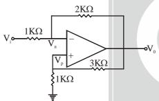
**Soln.** In the non-inverting loop applying KCL let  $V_p = V_n = V$
