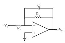
$$R_1 = 15.9 \text{K}\Omega, R_2 = 159 \text{K}\Omega, C = 1 \text{nF}$$
