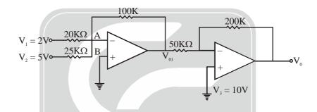
**Soln.** By VGP,  $V_B = V_A = 0$ , Now, KCL at point A,  $\frac{2}{20} + \frac{5}{25} = \frac{0 - V_0}{100} \Rightarrow V_{01} = -30Volt$
