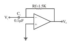
**Soln.**  $V_0 = -CR_f \frac{dV_i}{dt}$ ,  $V_0 = -0.1 \times 10^{-6} \times 1.5 \times 10^3 \cdot \cos(2\pi \times 10^2 t) \cdot 2\pi \times 10^2$
