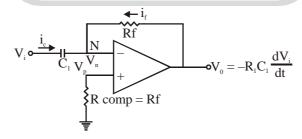
By VGP,  $V_p = V_n = 0$ , Now, KCL at point N,  $i_C = C_1 \frac{d}{dt} (V_i - V_N) = C_1 \frac{dV_i}{dt}$ , this is far capacitor current.
