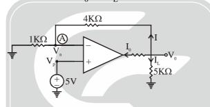
This is non-inverting amplifier.  $V_p = V_n = 5V$  by VGP. Soln. Now, KCL at point A
