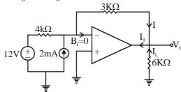
**Soln.** Applying KCL at point B,  $2 \times 10^{-3} + \frac{12}{4K} = \frac{0 - V_0}{3K}$
