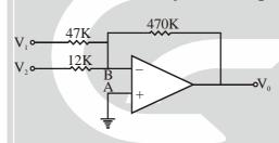
**Soln.**  $V_A = V_B = 0$ , Now applying KCL in inverting loop
