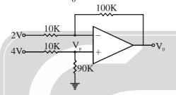
**Soln.** Firstly, considering first inverting loop,  $V_{01} = -\frac{R_f}{R_1}V_i \Rightarrow \frac{-100}{10} \times 2 = -20V$
