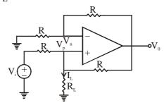
**Soln.** By VGP,  $V_n = V_p = V$ . Firstly, KCL in non-inverting terminal
