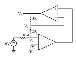
**Soln.**  $V_n = V_p = 0$ {VGP}, Now, KCL at point A,  $\frac{6-0}{3} = \frac{0-V_B}{2} \Rightarrow V_B = -4V$
