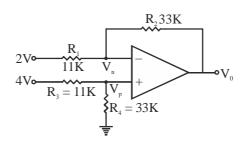
**Soln.**  $V_0 = 3(4-2), V_0 = 6 \text{ volt}$
