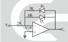
(i) If  $V_i = 3V$ , then  $V_0$ ? (ii) If  $V_i = -3V$ , then  $V_0$ ? **Soln.** (i) When  $V_i = 3V$ , diode  $D_1$  will on, Now KCL in  $D_1$  loop
