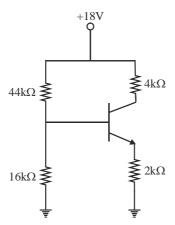
The value of the collectro-to-emitter voltage  $V_{CE}$  (in volts) is
