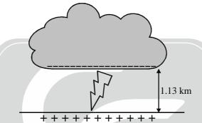
When the uniform electric field below the cloud reaches the value 2.4 MV m<sup>-1</sup> a lightning discharge occurs, and the entire charge of the cloud passes to the Earth below – which, in this case, behaves like a grounded conduc-
