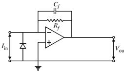
It is given that  $C_f = 100$  pF, and for  $I_{in} = 50$  nA D.C.  $V_{out} = 1$  V D.C. Therefore, the bandwidth of the above circuit is
