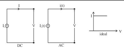
**Practical Current Sources:** Practical current sources delivers energy at specified current I, which is dependent on voltage across the source. In real time system current source does not exist.
