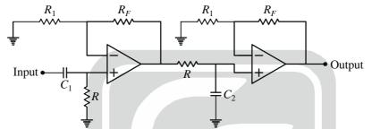
In order to get a lower cut-off frequency of 150 Hz and an upper cut-off frequency of 10 kHz, the appropriate values of  $C_1$  and  $C_2$  respectively are
