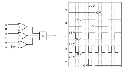
To obtain the output Y as shown in the figure, the logic gate X should be
