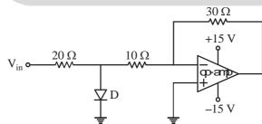
If  $V_{in}$  is a sinusoidal signal of frequency 50 Hz with an RMS value of 1 V, the maximum current that flows through the diode is closest to
