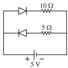
Given: The forward voltage drop across each diode = 0.7 V.
